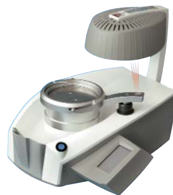
Figure 2. Thermoforming unit with foil temperature sensor system. The sensor in the base of the unit reads actual foil temperature; software programming and general operation is via the touchscreen on the right side of the machine.
