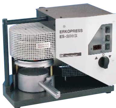
Figure 1. Typical Time based thermoforming unit: Note the simple control sequence and closed heating chamber to minimise atmospheric influences.
